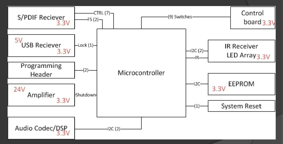
Next Step – start to build up current requirements for each device, and sum the current. DON'T FORGET LED CURRENT!
